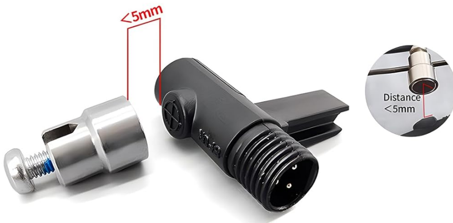
Figure 3.1: Visual guide for speed sensor installation, showing component assembly and optimal sensing distance.
