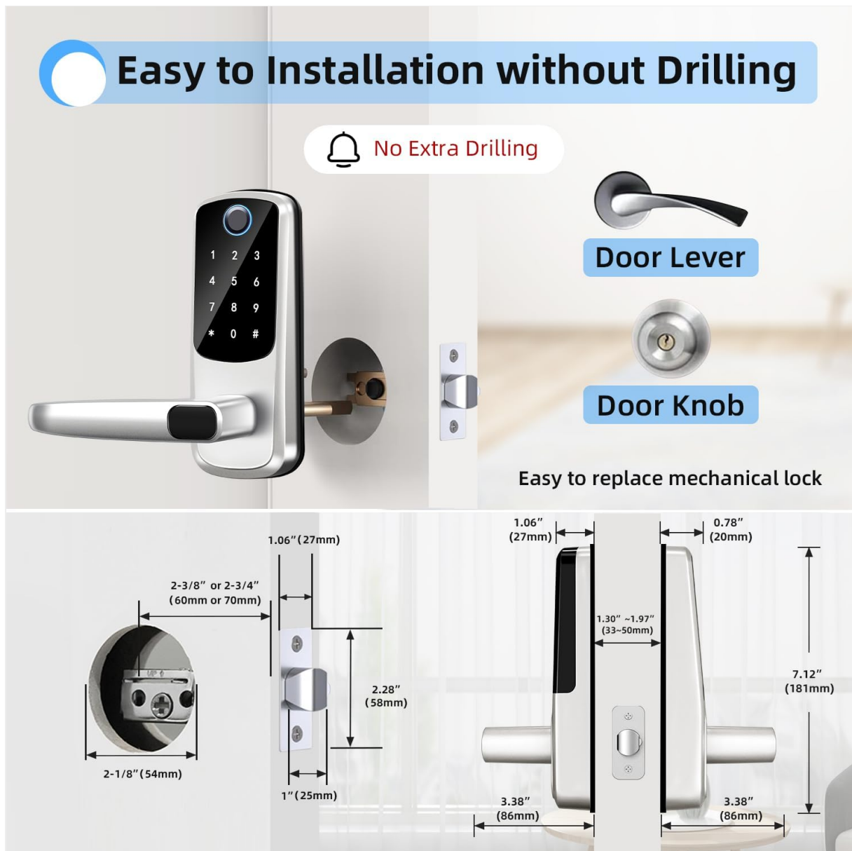
Figure 3.2: Installation Components and Dimensions
