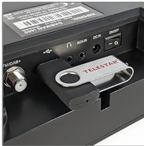
Figure 5.2: A USB stick inserted into the USB port on the back of the Imperial DABMAN i460, enabling media playback and recording.
