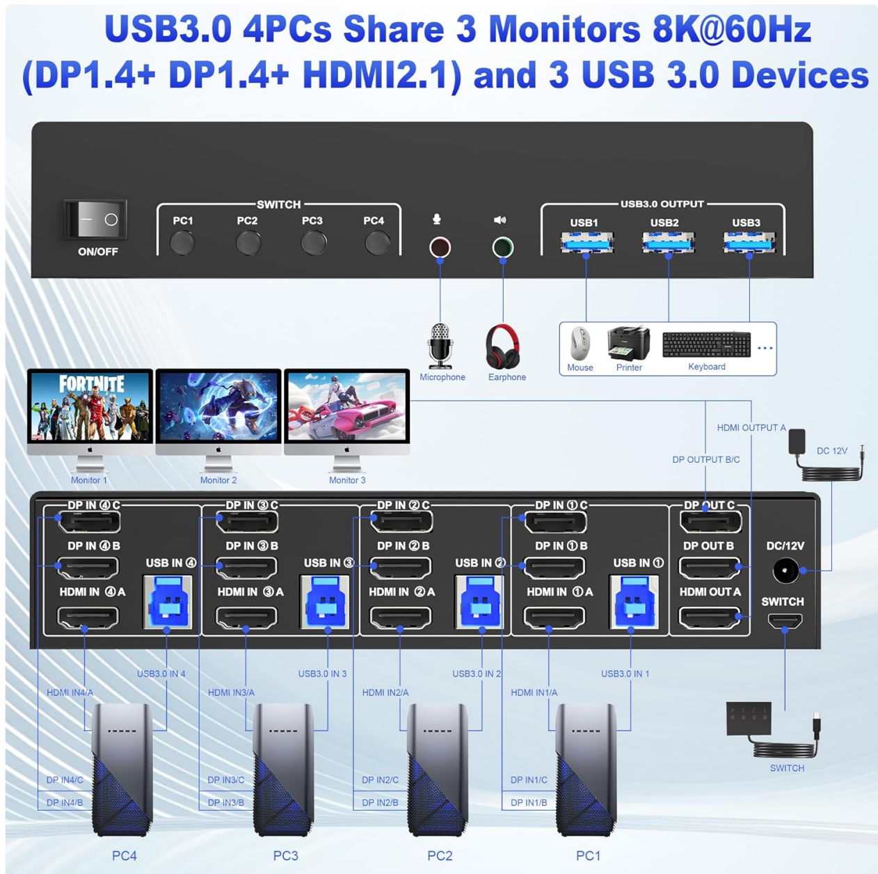
Image: Detailed diagram illustrating the connection points for computers, monitors, and peripherals on the KVM switch.
