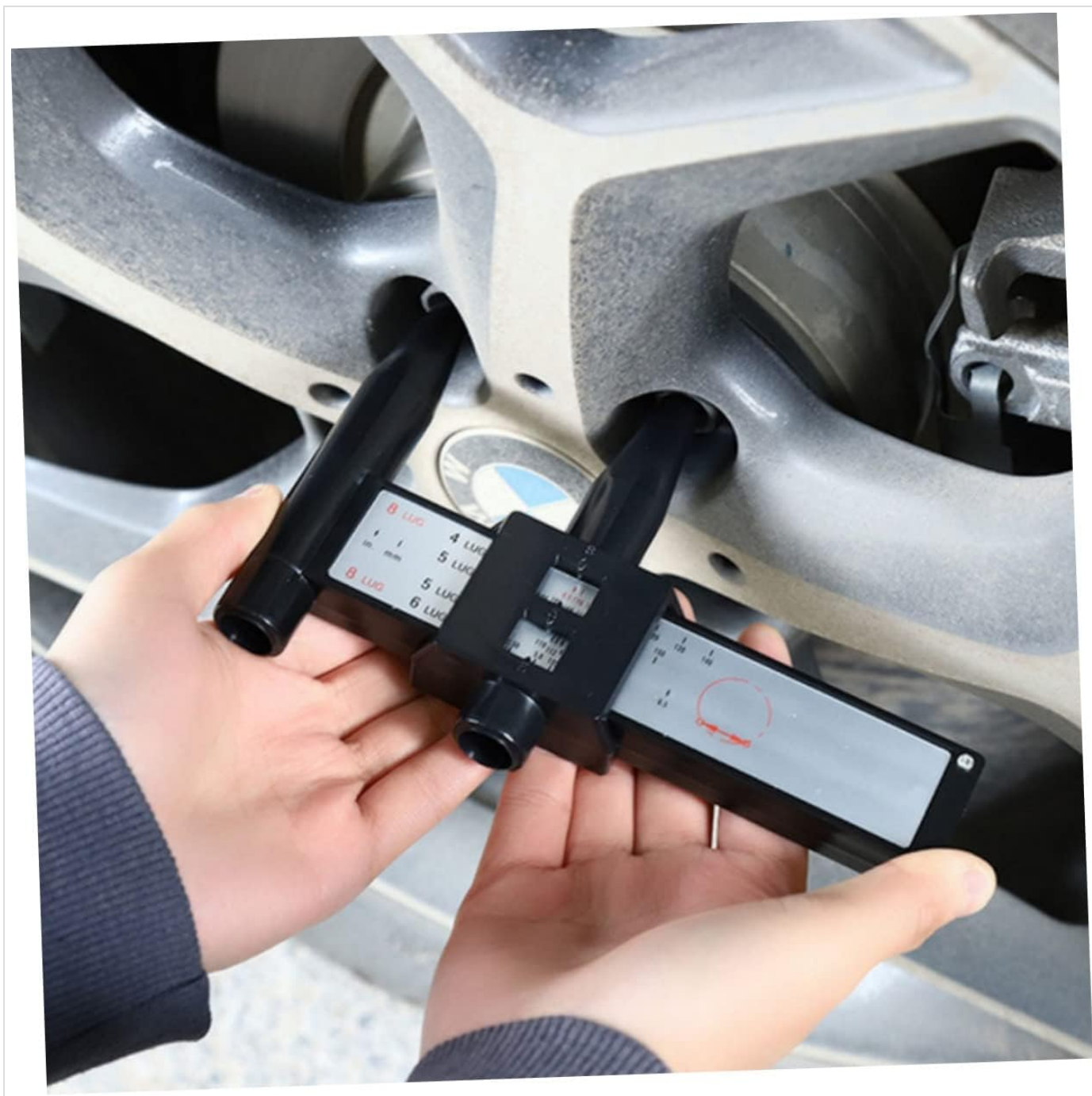
Figure 4: Close-up view of hands positioning the ruler to accurately measure a wheel's bolt pattern.
