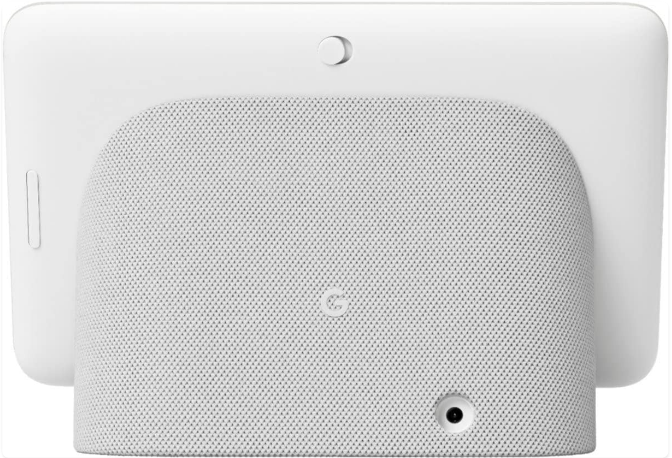
Figure 4: Rear view of the Nest Hub, showing the power input and the physical microphone toggle switch for privacy.
