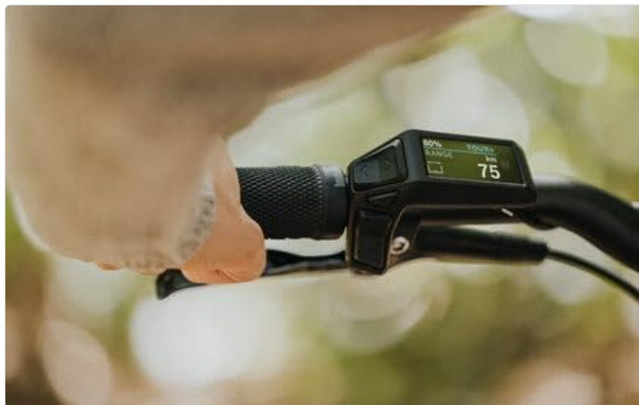
Image: A close-up view of the Purion 200 mounted on a handlebar, with a hand demonstrating how the thumb can easily reach the control buttons.
