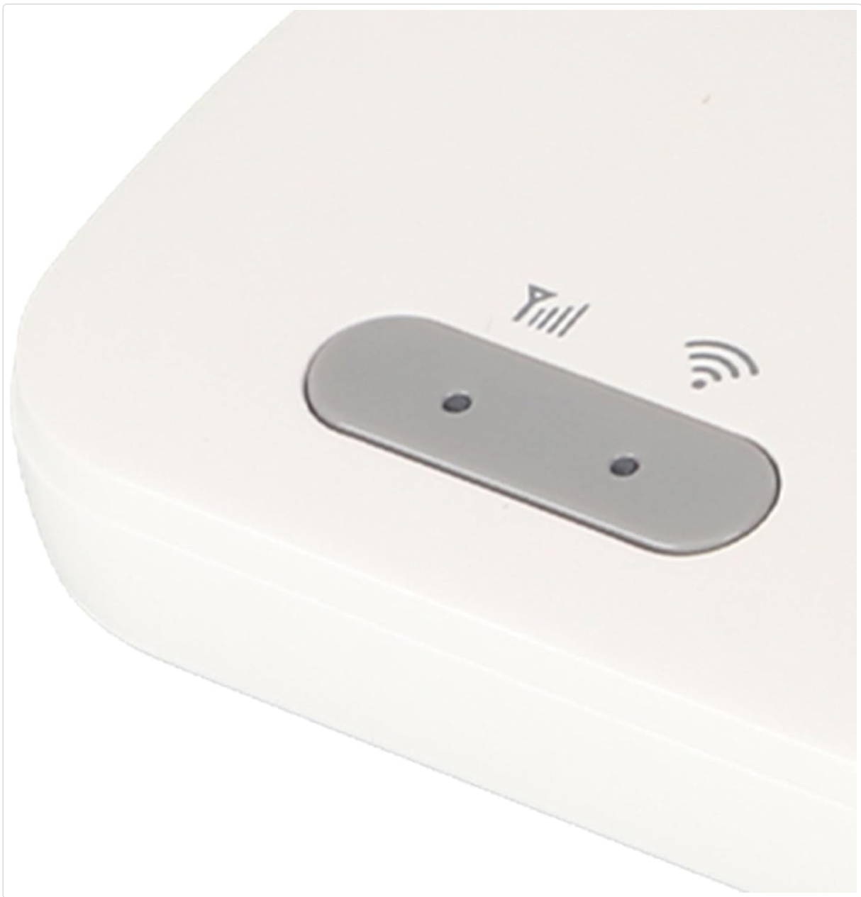
Figure 5.1: Indicator lights for signal and Wi-Fi status.
