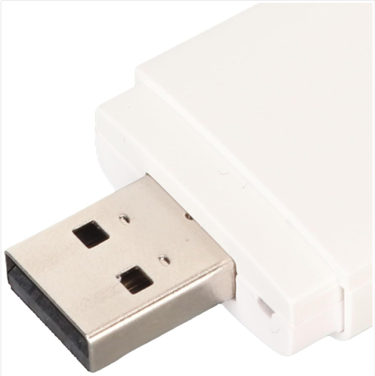
Figure 4.1: USB-A connector for power supply.
