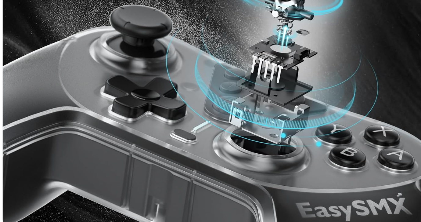
Figure 5: Hall Sensor Joystick Technology
