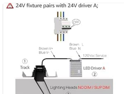
Image: Wiring diagram for connecting a 0-10V dimmable 24V driver to the track system.
