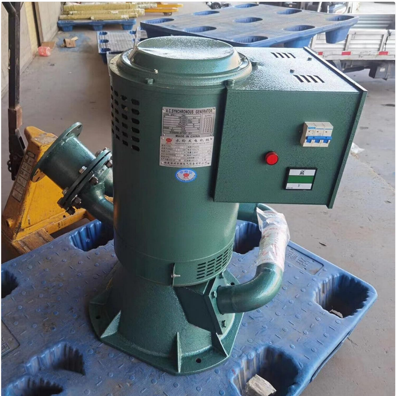
Figure 3.2: Side view of the OLONETO 30KW Single-Phase Hydraulic Generator, showing the integrated control panel. The control panel houses essential electrical components and user interfaces for operation.
