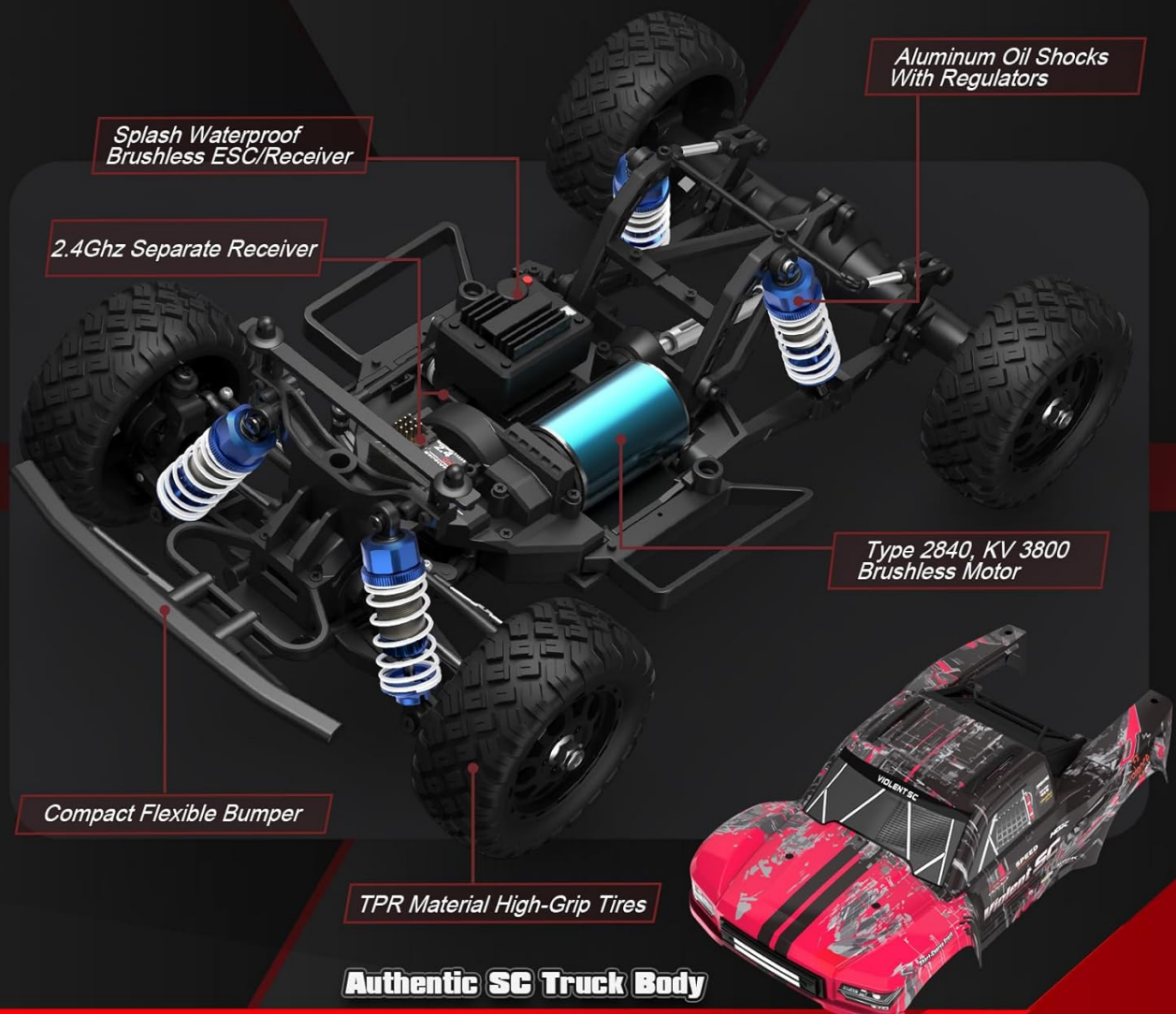
Image 4.1: Detailed view of the truck's chassis, highlighting the brushless motor, ESC, aluminum oil shocks, and high-grip tires.
