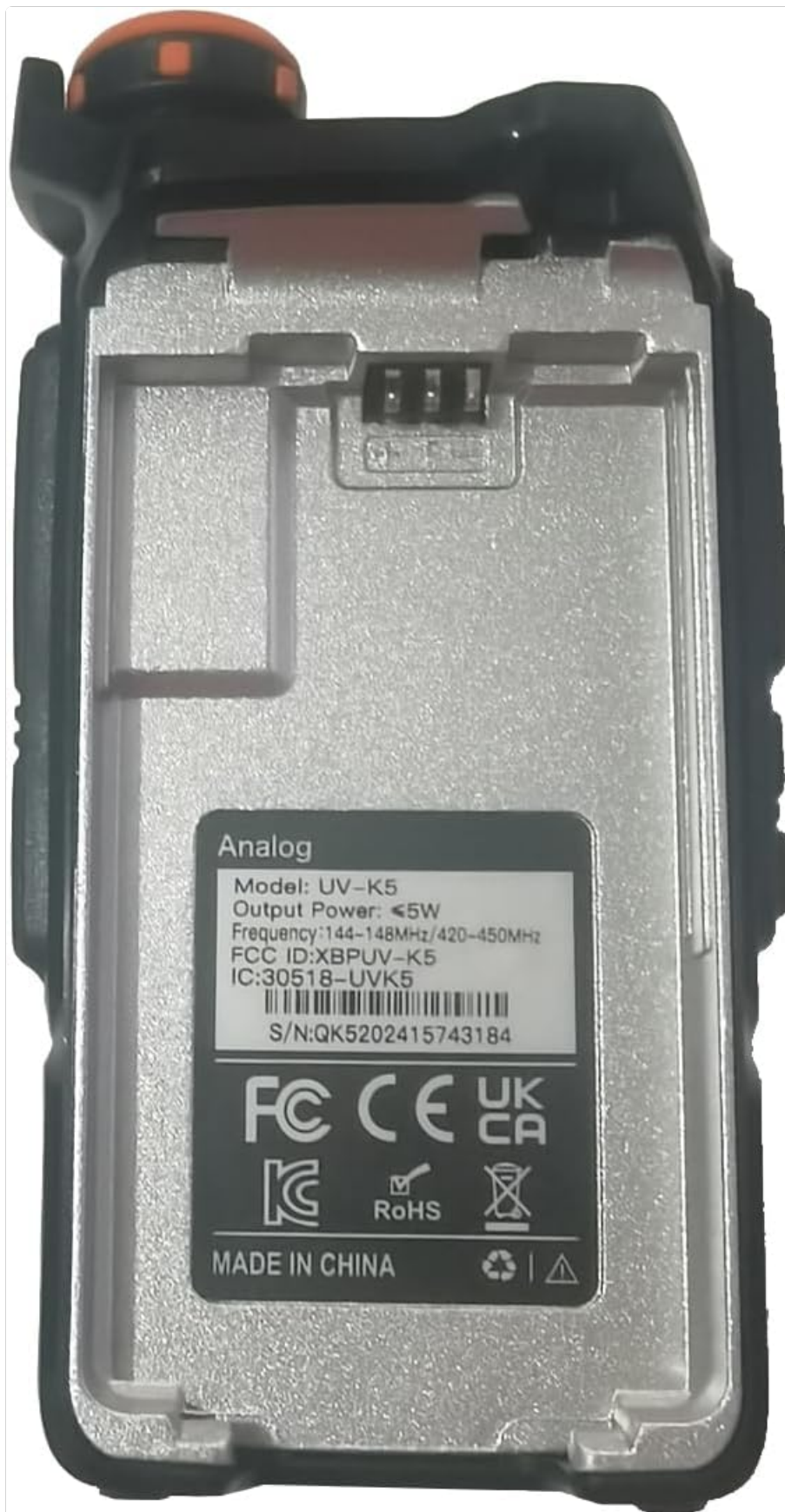
Figure 4.1: Rear view of the walkie talkie with the battery removed, showing the battery contacts and model information.
