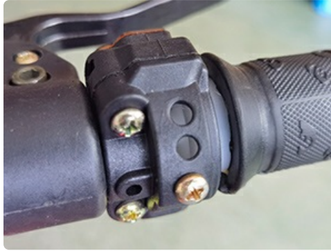
Image: Close-up of the adjustable throttle grip, which is part of the handlebar assembly.
