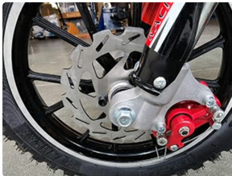
Image: Detailed view of the front disc brake assembly.
