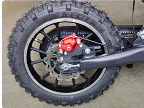
Image: Detailed view of the rear wheel and disc brake, important components for regular inspection.
