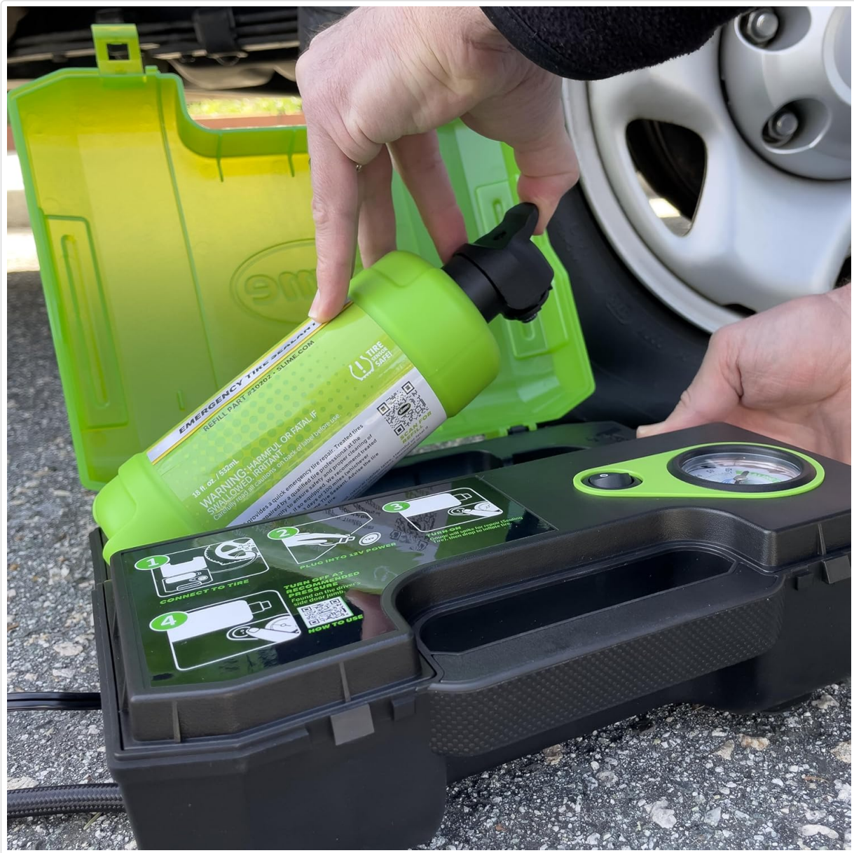
Image 5: A hand inserting a new Slime sealant bottle into the tire repair kit, aligning it correctly.
