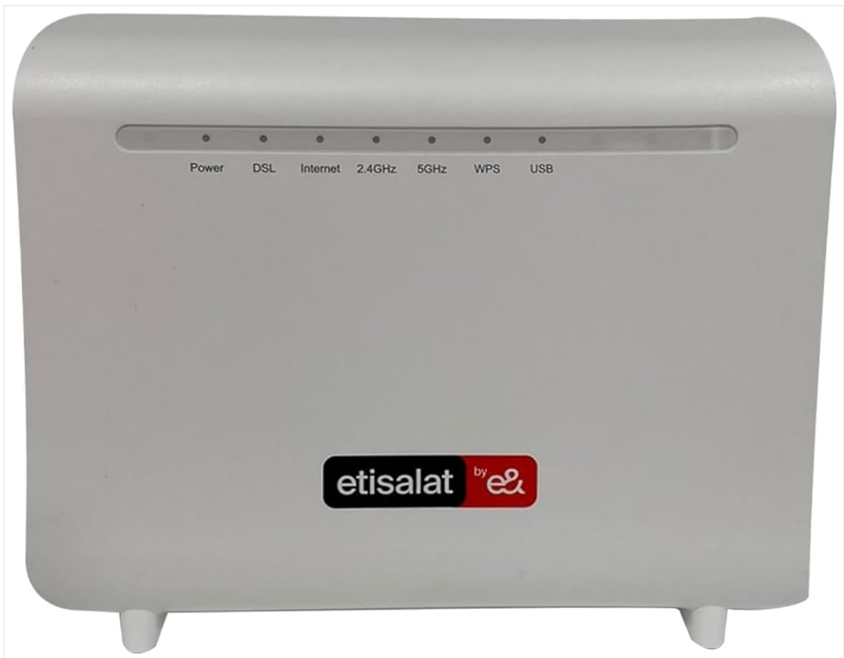
Figure 1: Front panel of the ZTE ZXHN H188A VDSL Router. Visible indicators include Power, DSL, Internet, 2.4GHz Wi-Fi, 5GHz Wi-Fi, WPS, and USB. The lower front features the 'etisalat by e&' logo.
