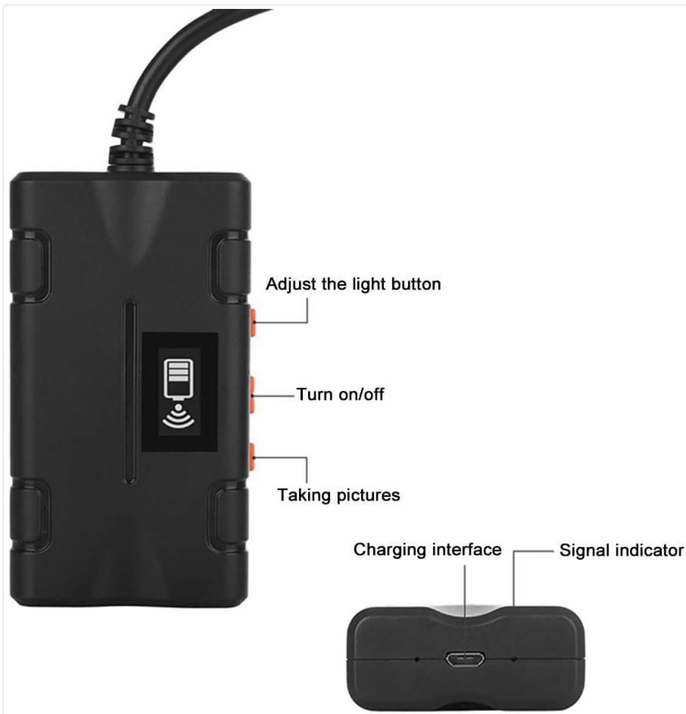
Figure 4.2: Control unit with labeled buttons and charging interface.
