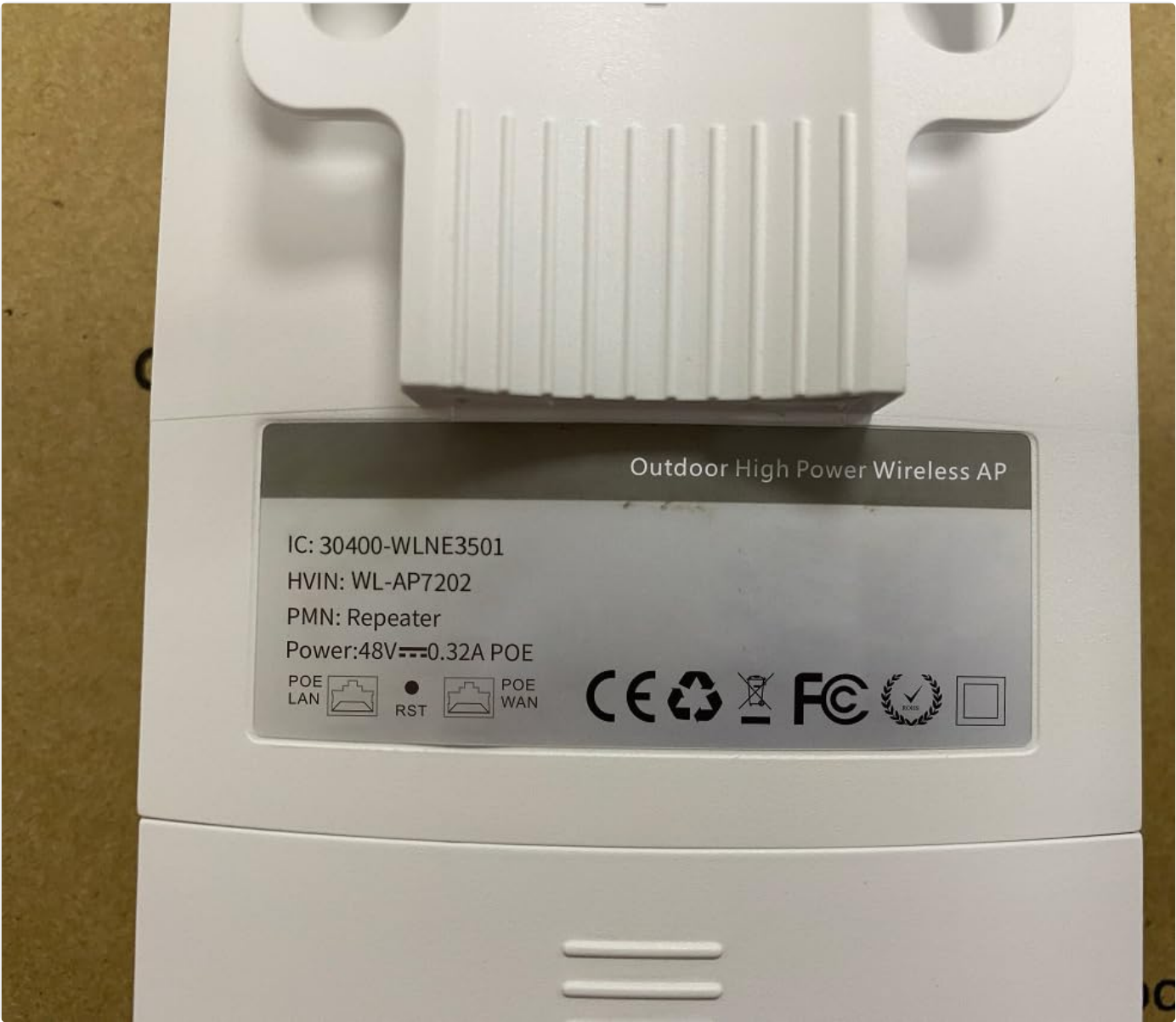
Figure 6.1: Back label of the device, displaying model number (WL-AP7202) and power specifications (48V PoE).
