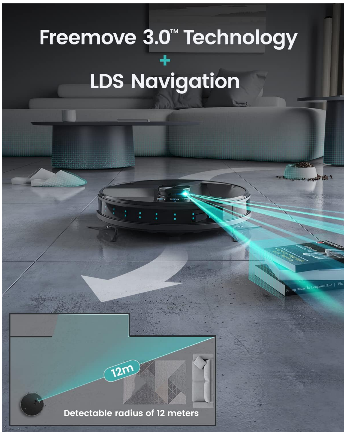
Image 3.3: The LS1 utilizing its LDS navigation system to detect its surroundings, with a detectable radius of 12 meters.
