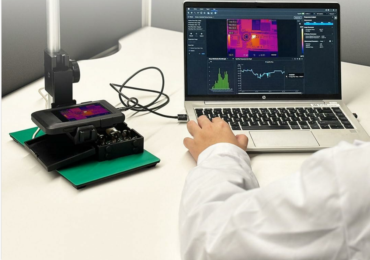
Figure 3.9: The HIKMICRO PocketC camera set up with a clip-on macro lens, demonstrating its ability to take temperature readings on small objects like components on circuit boards.
