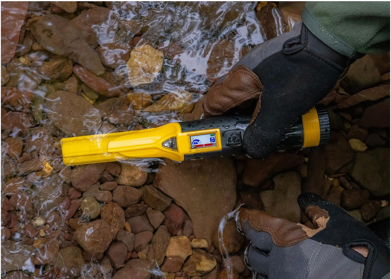
Image: The Nokta AccuPoint Pinpointer being used underwater, showcasing its waterproof design for aquatic treasure hunting.
