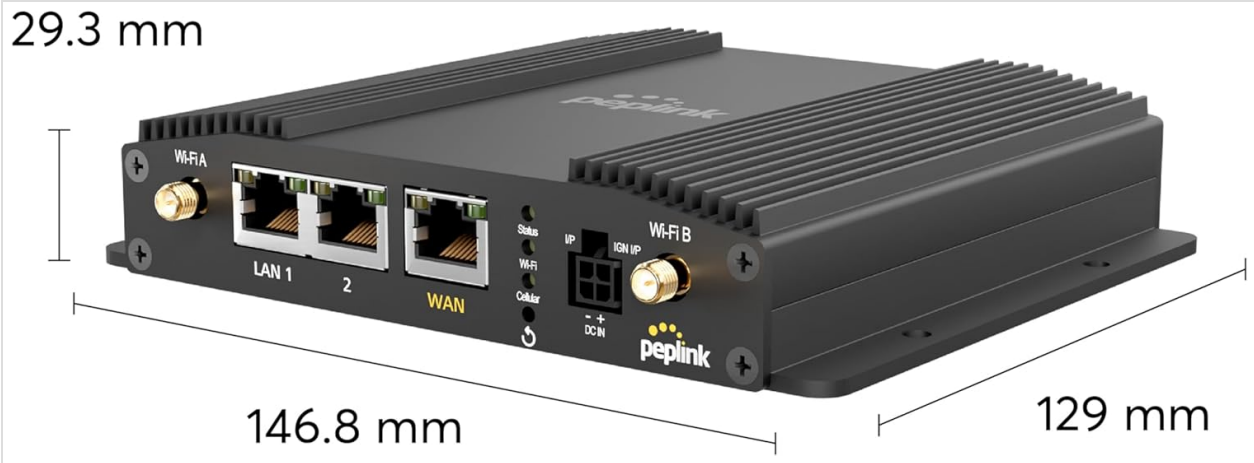
Image: Side view of the Peplink MAX BR1 Pro 5G Router, showing its compact dimensions of 146.8 mm length, 129 mm width, and 29.3 mm height.
