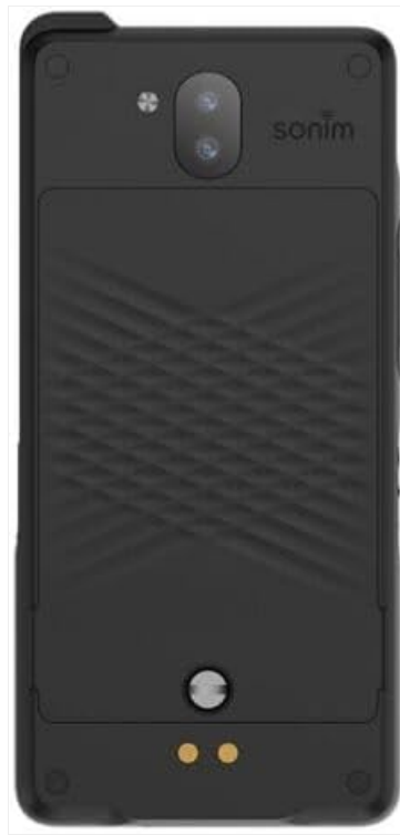
Image 2.1: Rear view of the Sonim XP10 smartphone, showing the camera module and charging contacts.
