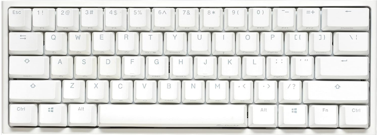
Image: A full top-down view of the Ducky One 2 Pro Mini keyboard, showing the compact 60% layout and secondary function legends on the keycaps.
