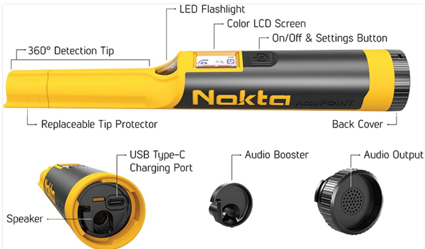
Figure 2: Labeled components of the AccuPOINT Pinpointer.
