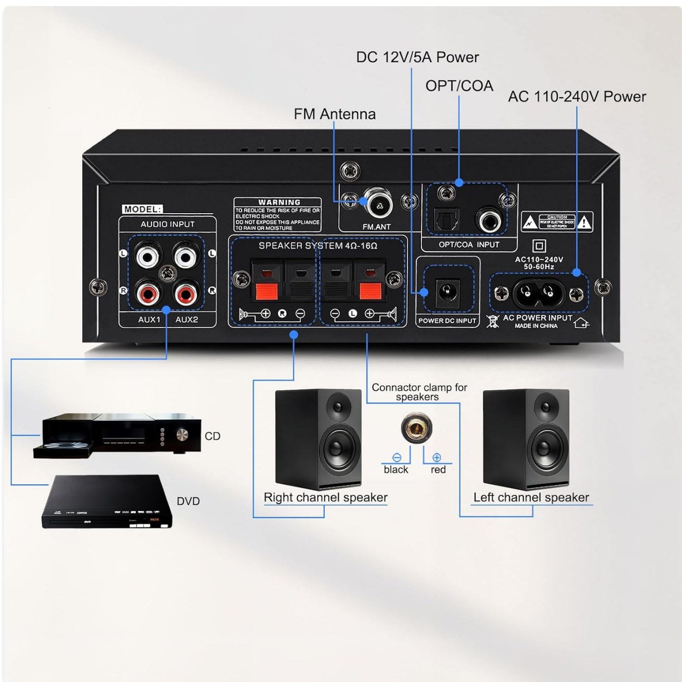
Rear panel connections for the AK55 amplifier.
