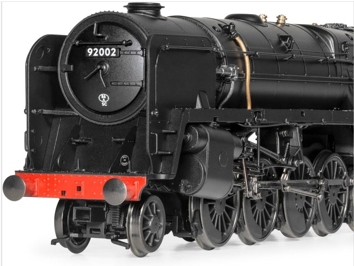
Image 3: Side view of the Hornby R30132 BR Class 9F locomotive, showcasing the 2-10-0 wheel configuration and detailed valve gear.
