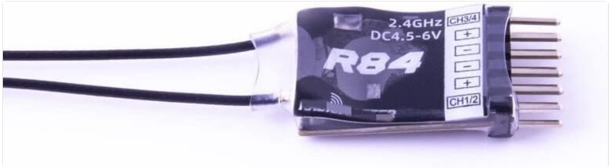
Image: Radiomaster R84 4CH Receiver, showing its compact size and pin configuration for channels 1-4 and power input.
