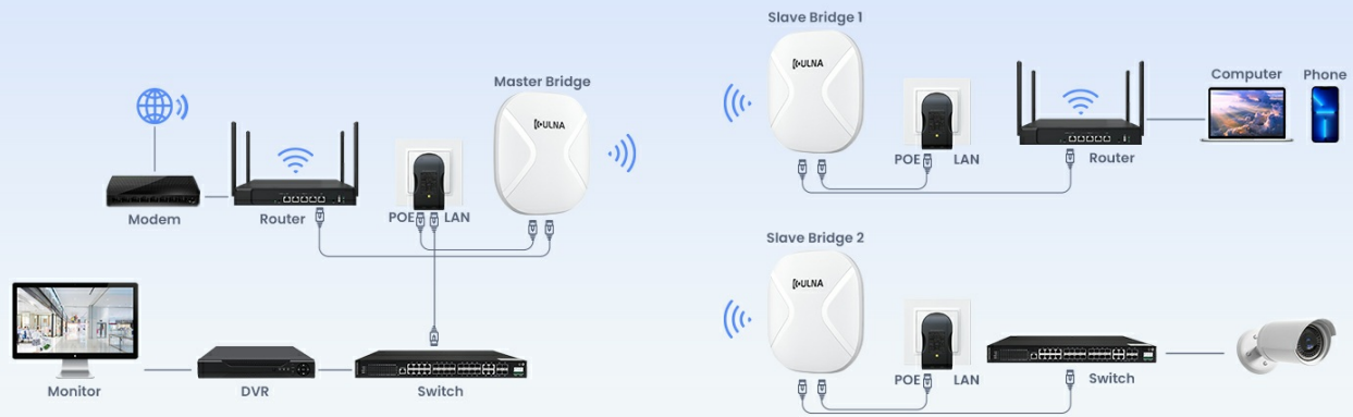
Figure 5.2: A detailed example of a Point-to-Multipoint setup, connecting multiple remote devices via Slave Bridges to a central Master Bridge.
