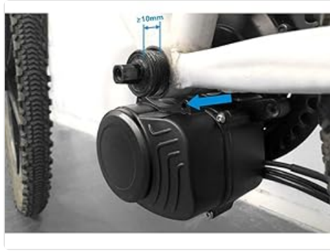
Image 5.5: During speed sensor installation, aim for the arrow position of the product to ensure a 10mm distance between the speed sensor and the magnet.
