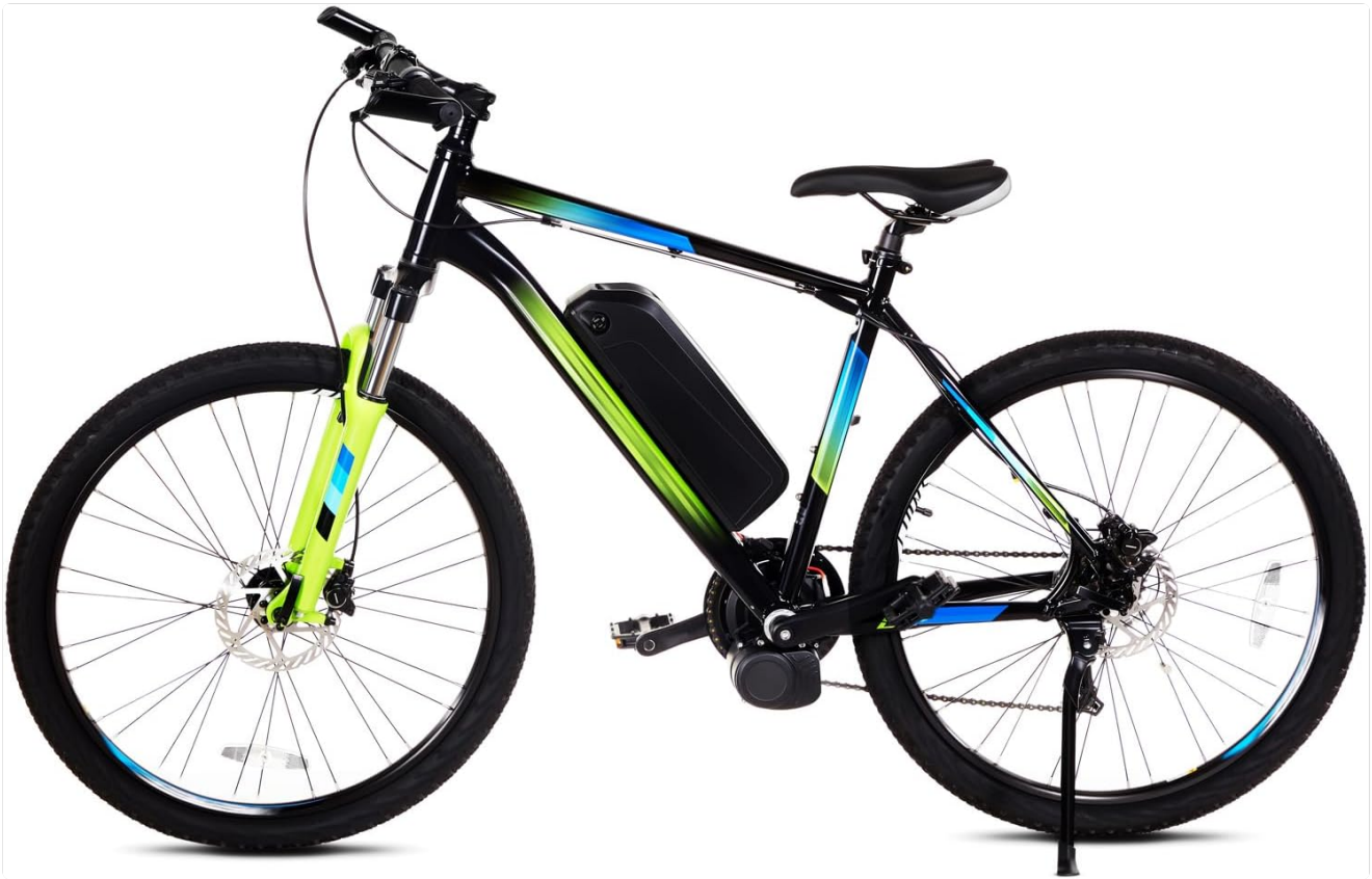
Image 1.2: An example of a bicycle converted with the TSDZ2B mid-drive motor kit.
