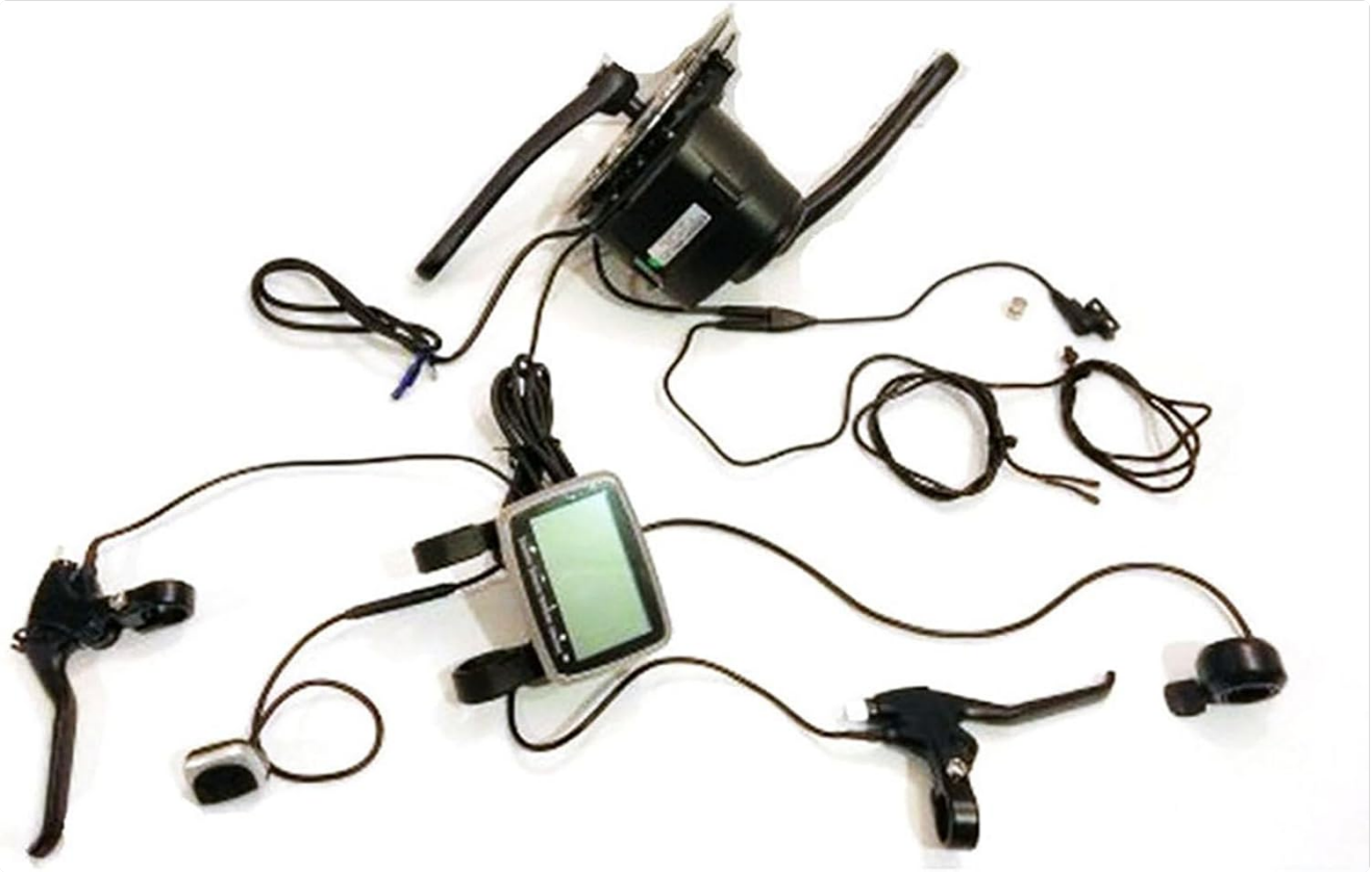
Image 3.2: All included components of the TSDZ2B kit, including the motor, display, brake levers, throttle, and cables.
