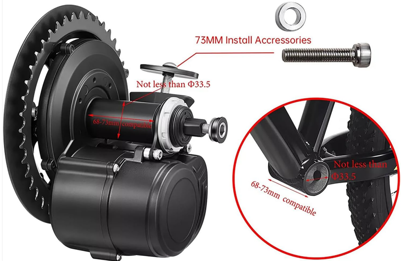
Image 5.1: Diagram illustrating bottom bracket compatibility requirements (68-73mm width, >33.5mm inner diameter).
