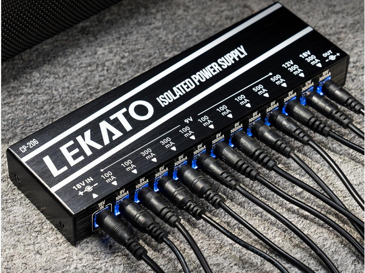
Image 7.1: The power supply's individual short-circuit protection ensures other pedals remain operational.
