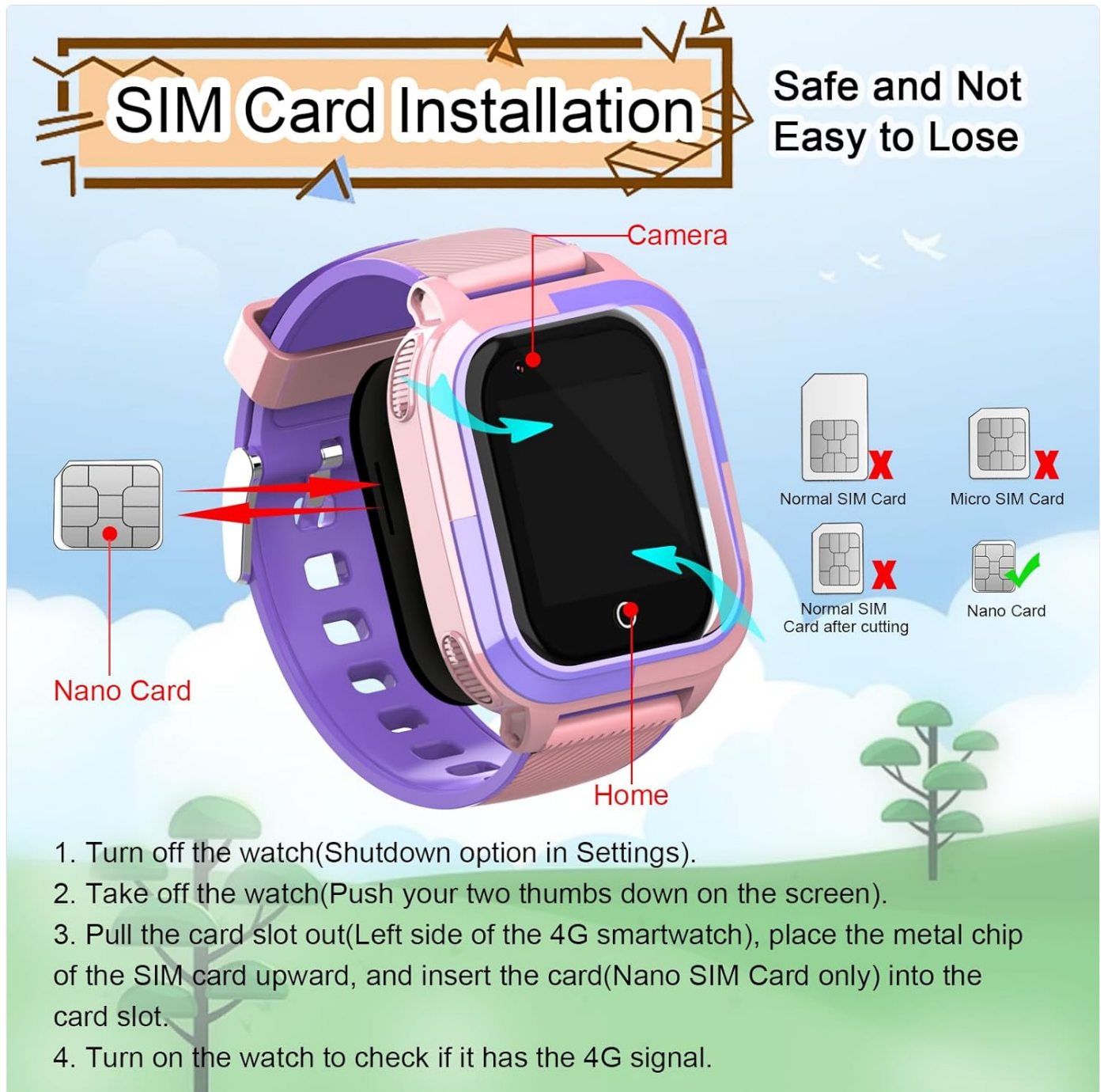
Image 4.2: Visual guide for Nano SIM card installation.
