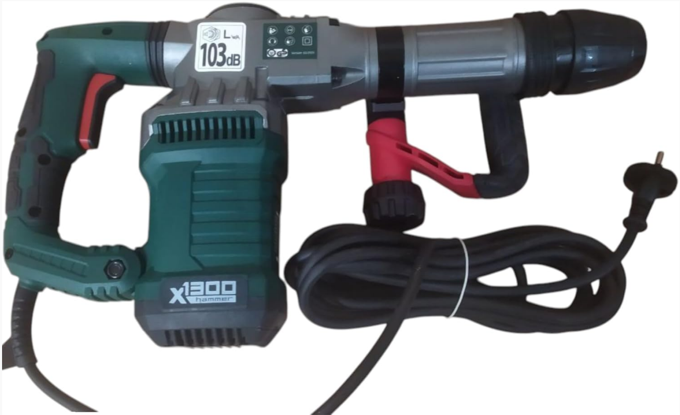
Side view of the demolition hammer, highlighting the SDS-Max chuck and the ergonomic design of the handles. The power cord is visible coiled next to the tool.
