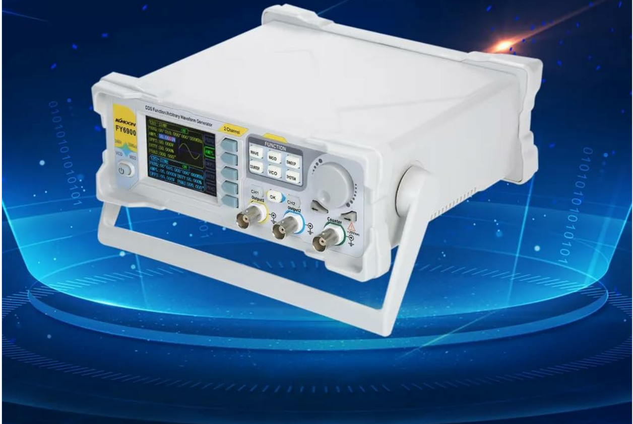
Figure 2.3: Key features of the Digital DDS Dual-channel Signal Generator. This image displays the 2.4-inch TFT Color LCD with 320x240 resolution, 250MSa/s sample rate, 0.01S-999S sweep time, 1mVpp-24Vpp amplitude, and 8192 points * 14bits waveform length.
