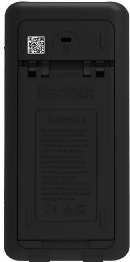
Figure 2: Rear view of the Hantek 2D42 showing the battery compartment and Type-C charging port. The device uses 18650 replaceable lithium batteries.
