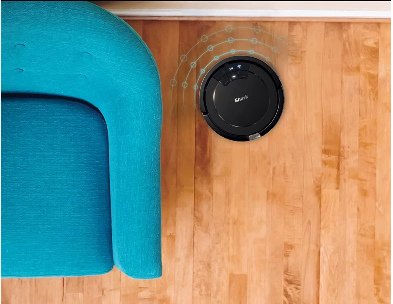
Figure 3: Robot avoiding obstacles with bumper sensors.
