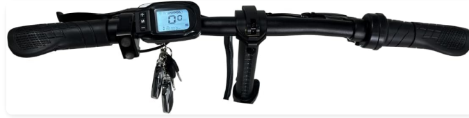
Image 5.1: Close-up of the handlebars, showing the display and control buttons.
