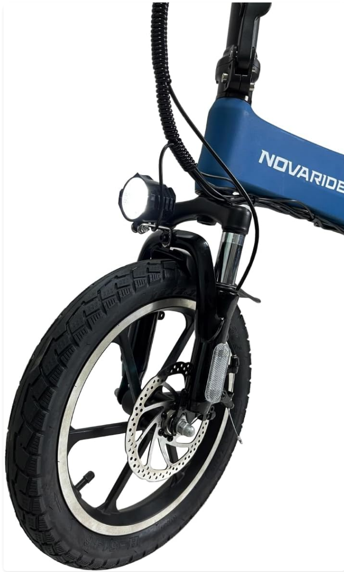
Image 5.2: Close-up of the front wheel, showing the disc brake and headlight.
