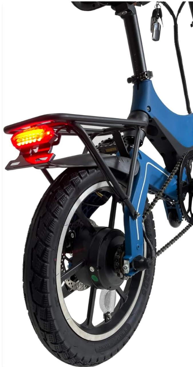
Image 5.3: Close-up of the rear wheel, motor, and taillight.
