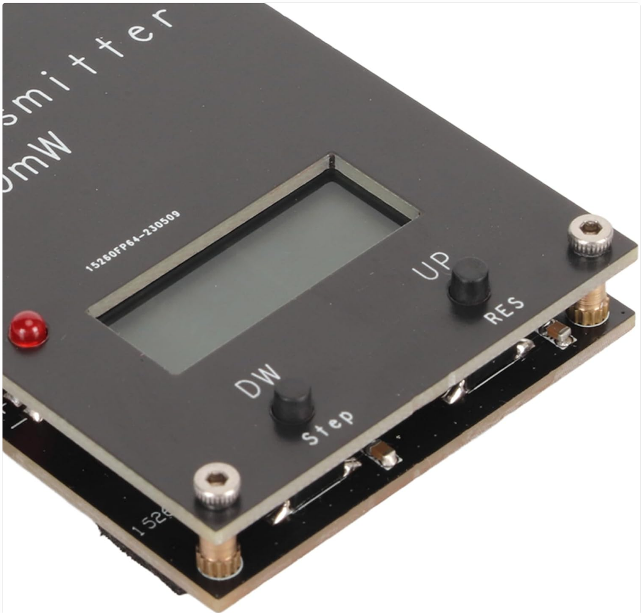
Image: The control buttons (UP, DW, RES) and LCD screen on the ASHATA FM Transmitter.
