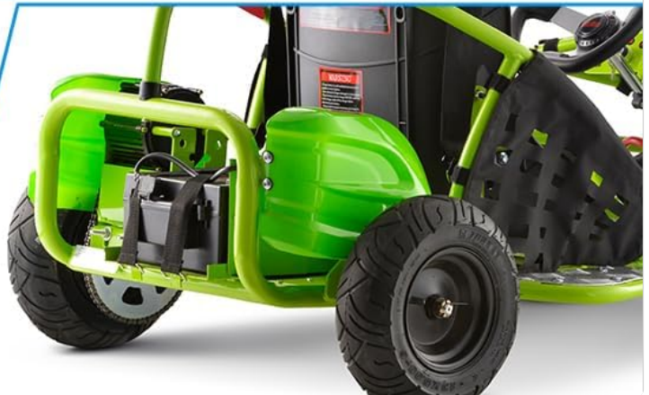
Image 8.1: Go Kart Components. This image details the go-kart's steel tubular frame, 13-inch pneumatic tires, 1000W brushless motor, and 48V 12Ah battery.
