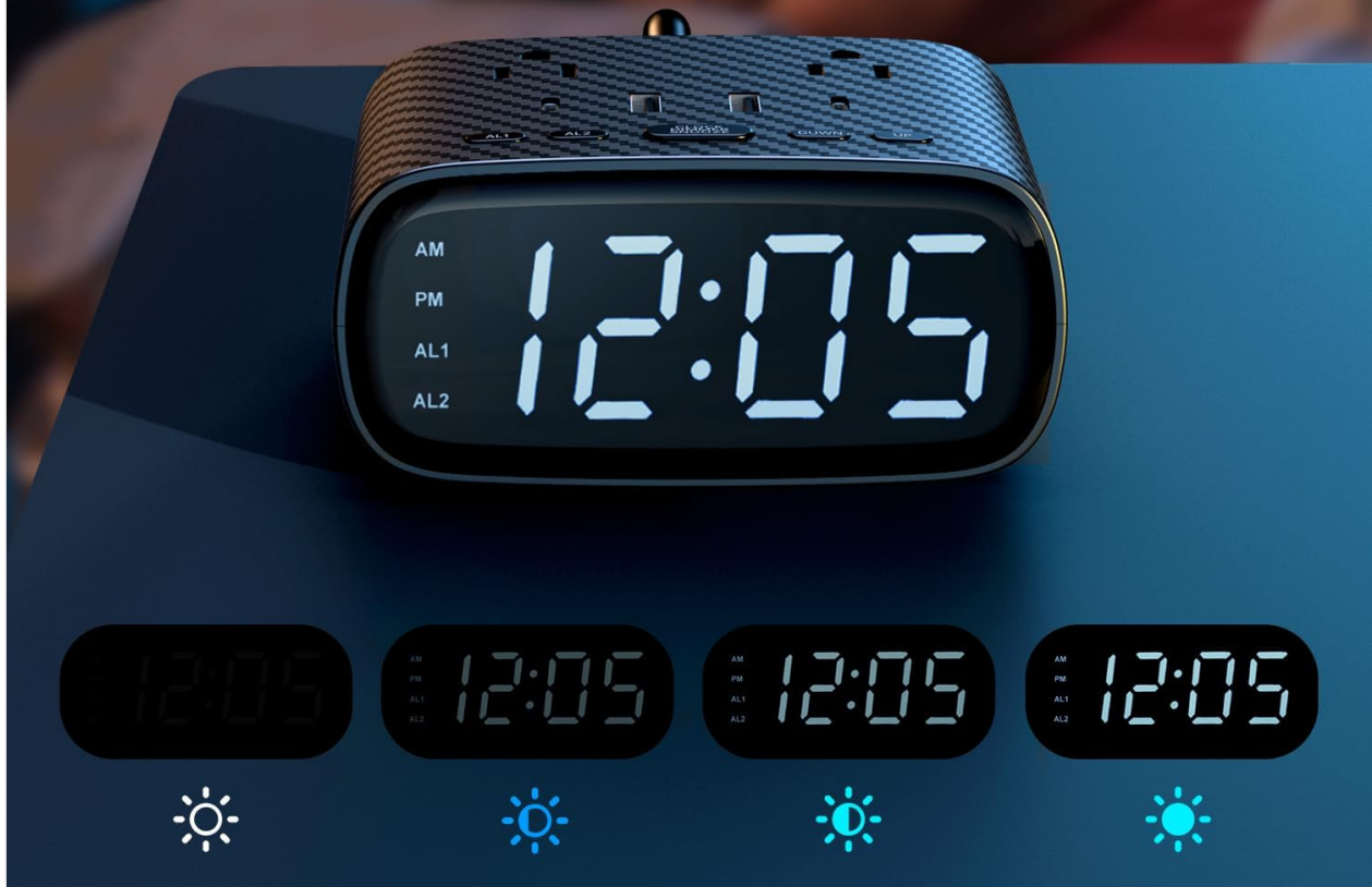
Figure 2.3: Illustration of the 4-level dimmable LED display, showing various brightness settings.
