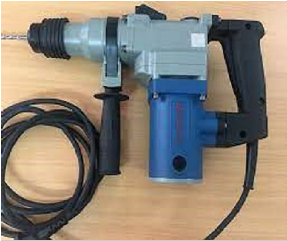
Figure 6.1: The Dongcheng DZC03-26B Demolition Hammer, showcasing its main body, handles, and attached power cord, ready for connection to a power source.
