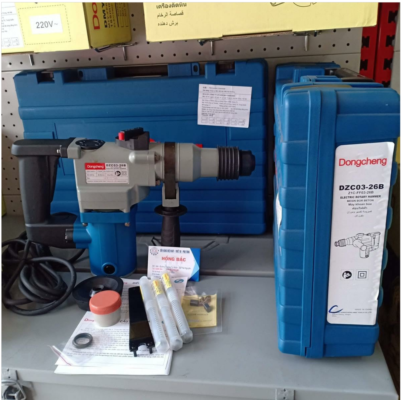
Figure 3.2: The Dongcheng DZC03-26B Demolition Hammer displayed with its full set of accessories, including drill bits, chisels, and the carrying case.
