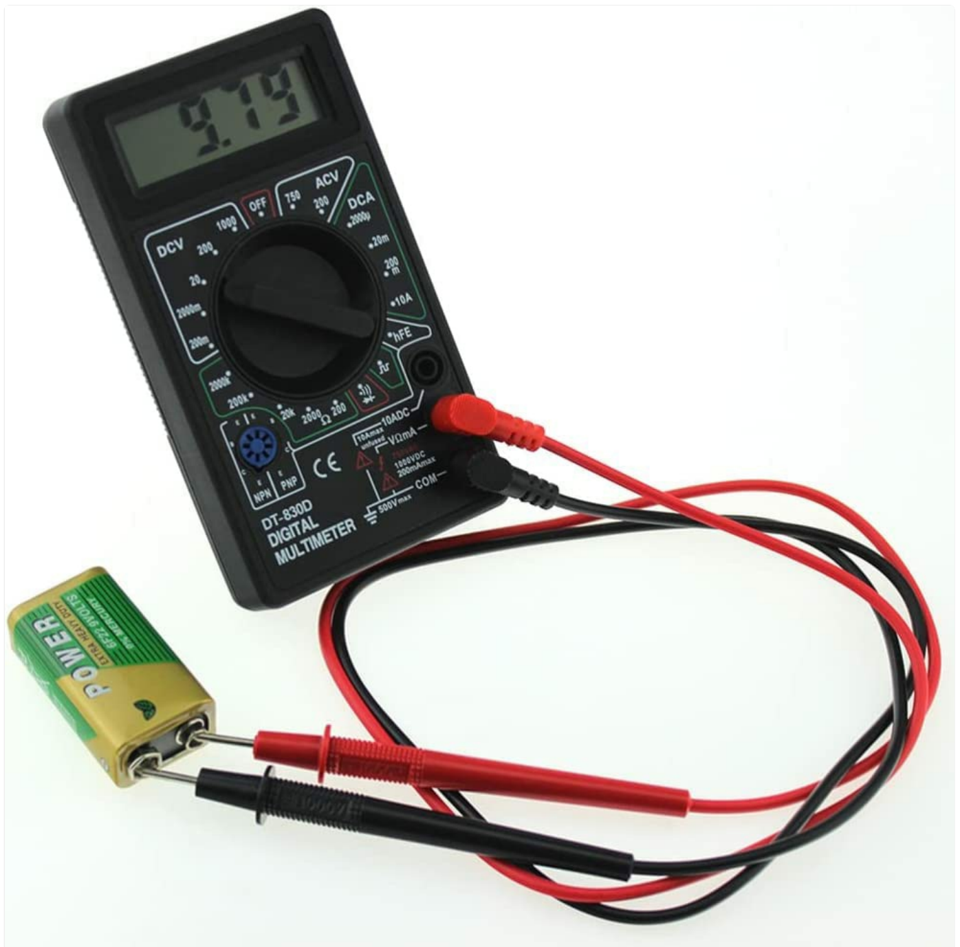
Image: The DT-830D Digital Multimeter with its test leads connected to a 9V battery, demonstrating a DC voltage measurement in progress.
