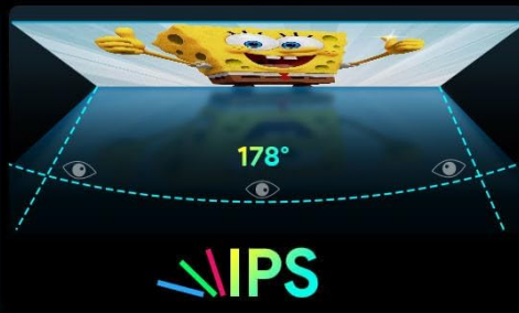
Image 3.1: The QLED IPS screen offers a new level of clarity with brilliant details and colors, featuring a 178° wide viewing angle and responsive capacitive touch.
