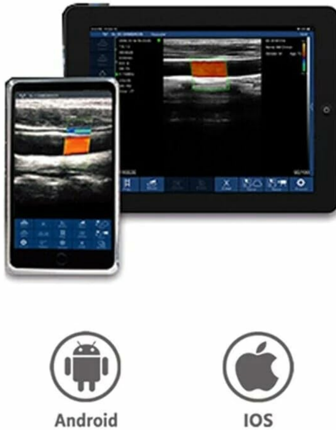
Figure 3.2: The ultrasound software running on a smartphone and tablet, compatible with Android and iOS. Once the software is installed, power on the ultrasound device. The device will broadcast a WiFi signal. Connect your mobile device or computer to this WiFi network. The effective transmission distance for the WiFi connection is approximately 10 meters in an open area.
