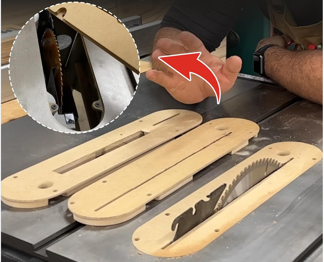
Figure 4.1: The installation process, which may involve minor sanding for a perfect fit.
