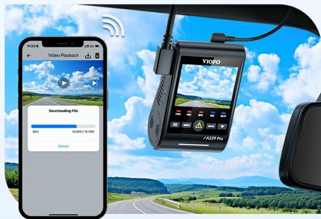
Control your dash cam hands-free with 12 voice commands, including 'take photo', 'lock the video', 'turn on WiFi', and 'show front/rear camera'. The dash cam also provides clear voice notifications for setting changes or memory card errors.
