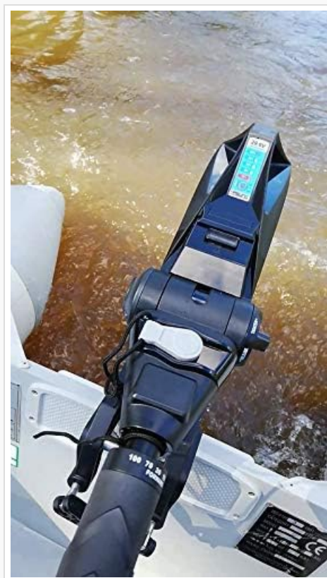
Figure 5.1: Control Handle and Display. This image provides a top-down view of the motor's control handle, clearly showing the integrated digital display with battery and power indicators.
