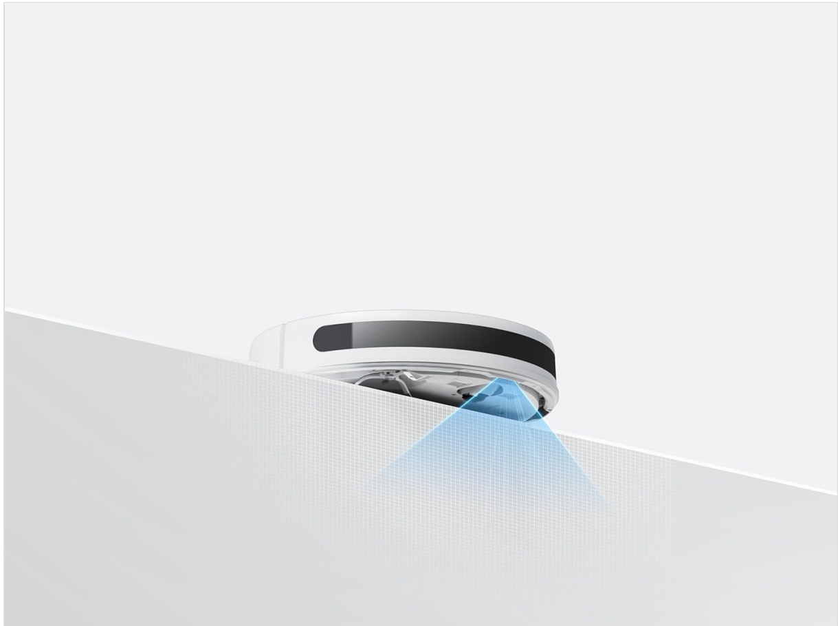
Figure 7: Diagram illustrating the function of the cliff sensors, which prevent the robot from falling down stairs or off ledges.
