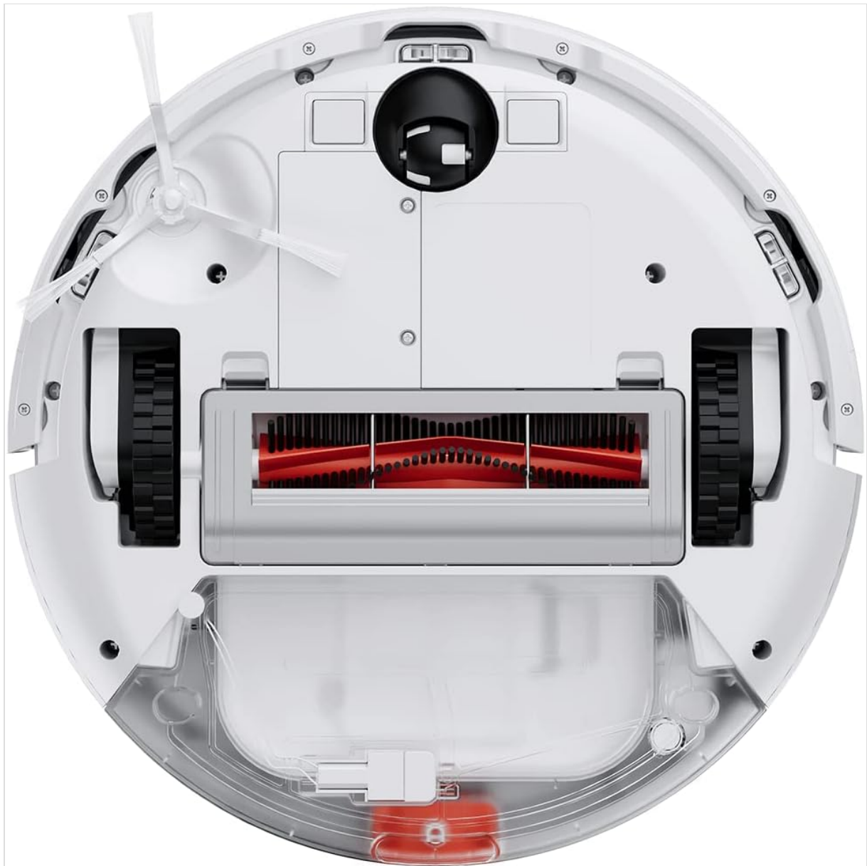
Figure 3: Underside of the robot vacuum, showing the main brush, side brushes, wheels, and dustbin/water tank compartment.
