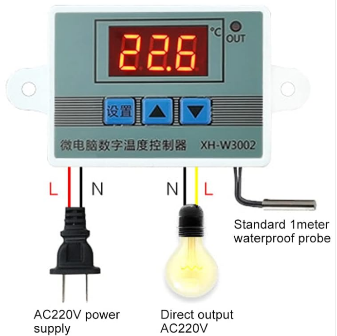
Figure 4.1: Wiring diagram for the XH-W3002. Ensure to use the correct wiring for your power supply (DC12V/24V or AC220V).
