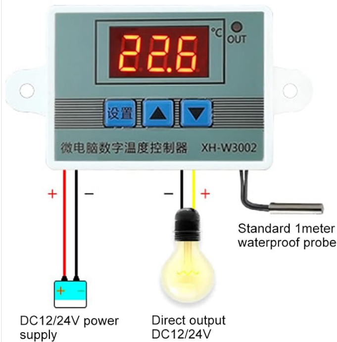
Figure 4.1: Wiring diagram for the XH-W3002. Ensure to use the correct wiring for your power supply (DC12V/24V or AC220V).
