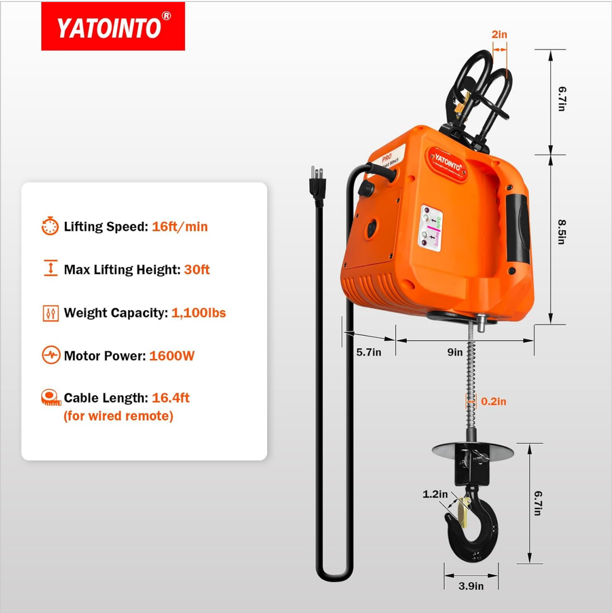
Figure 4.1: Detailed dimensions and key specifications of the YATOINTO PRO Electric Hoist Winch 1100LB.
